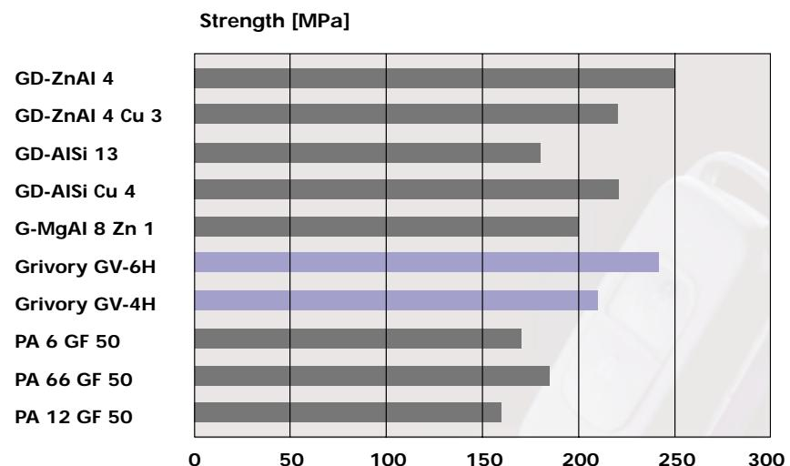
Plastic in a conditioned state according to ISO 1110, metals according to DIN 1743, 1725, 1729, 9715
