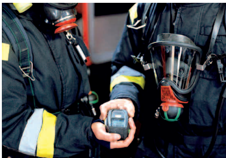
Fig. 4. Two-component safety mask of high-performance polyamide with all-round rubber sealing
